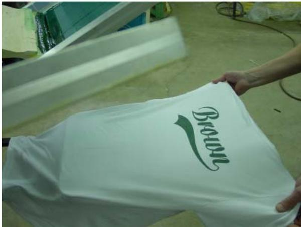
The flash unit should be set on “high” and be approximately 3” away from the garment. It will take anywhere from 5 to 20 seconds to flash an ink. Remember that you are not trying to cure the ink on the shirt. Over flashing will cause its own list of problems
