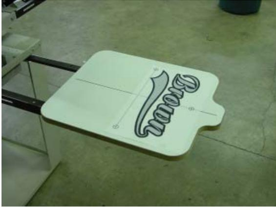
4. Bring the first screen down to the platen. Move it around until the registration marks on the screen match the marks on the MAP. When it does tighten the screen clamp knobs to secure the frame.
